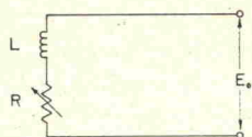
FIG. 4. Equivalent circuit of current supply when current path is through the inductor and gauge plus terminating resistors.
